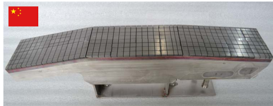
Enhanced Heat Flux Panel, tested at: 4.7 MW/m 2 for 7500 cycles 5.9 MW/m 2 for 1500 cycles
